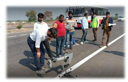
road markings on public roads in Ireland should be Class S2 SRT > 50. The skid resistance of freshly applied road markings tends to increase in value due to the effects of trafficking and weathering. For items such as transverse yellow bar markings at roundabouts, hatching and chevron areas, a higher Class of skid resistance is generally specified.
